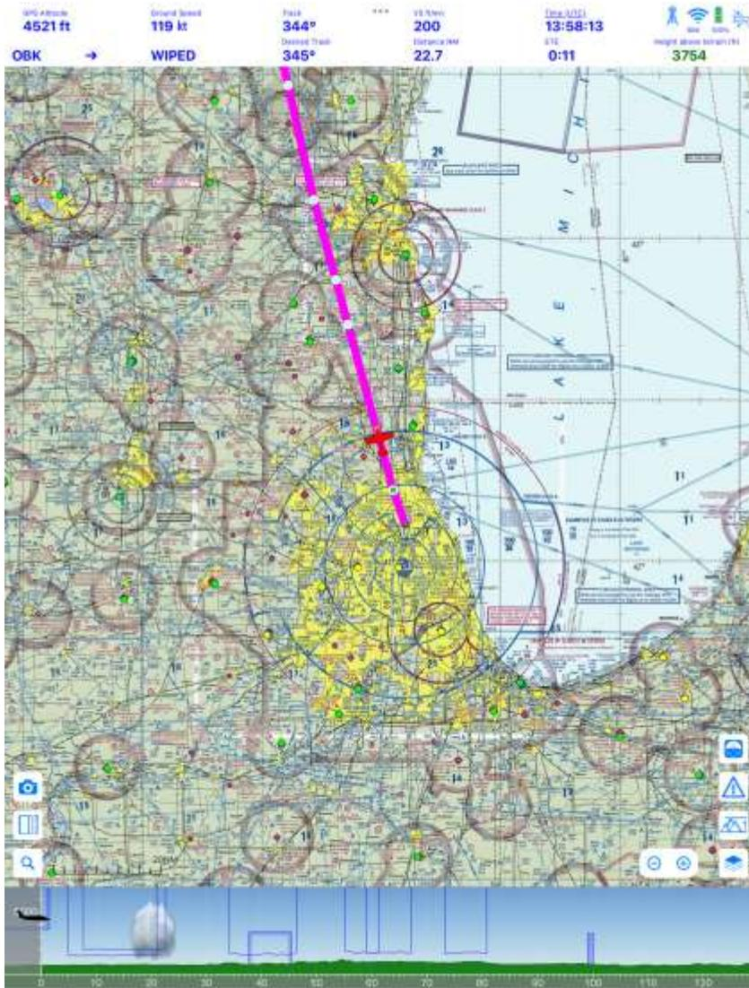
**Flight mode** requires GPS position information. Position data may be provided by the internal GPS of the device or from an external GPS that may provide a better accuracy and will lower the device current draw. Please note that iPads without mobile connectivity do not have embedded GPS and will require an external device. Please refer to the Appendix B regarding supported external GPS.
