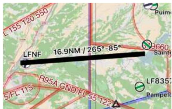
In addition, a long press with two fingers on two different locations on the map will display a temporary black ruler showing course (both directions) and distance between those points.
