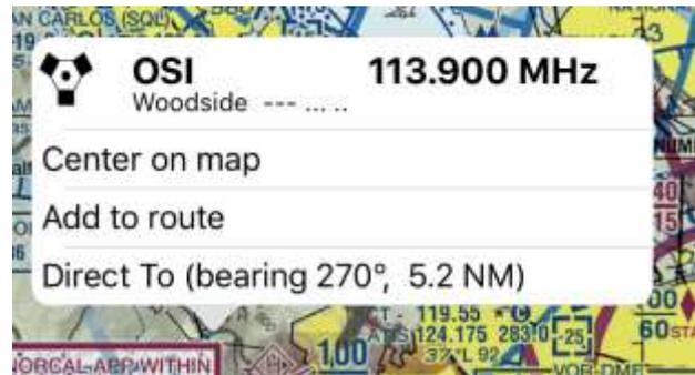
It is possible to end the **Direct To** mode and revert to normal navigation along the planned route by clicking again on the direct to point and selecting **End Direct To** mode.
