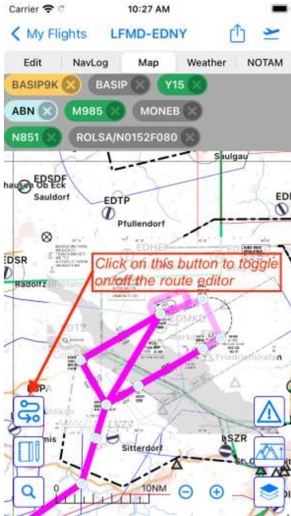
You could toggle the route editor display on top of the aviation map, either on the ground or during flight, thanks to the route button
