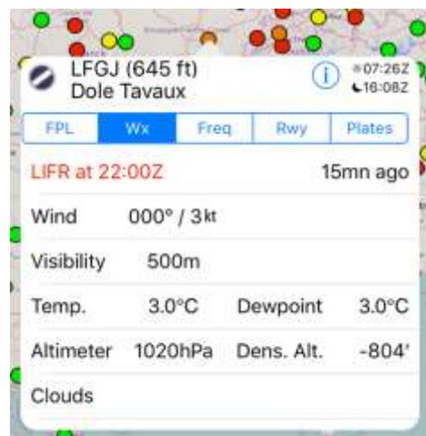
information such the computation of the airfield density altitude. Scrolling down this weather window will display the raw METAR and raw TAF. This airport detail window allows also to view the other airfield data (frequencies, runways, plates).
