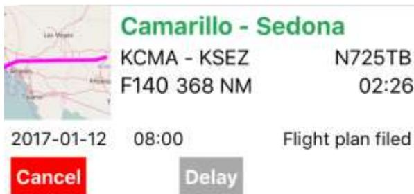
It is recommended to use Delay instead of Cancel and filing again, because this avoids using another flight plan token for filing. It is not authorized to advance the flight time in AFTN network, so if you may be able to takeoff earlier than planned, it is best to file the plan with an earlier time and delay it, otherwise a Cancel / File again operation will be needed to advance flight time.
