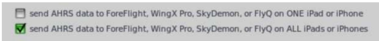
The first option with broadcast aircraft data to your whole Wi-Fi network, your router should transmit them to your iPhone/iPad device. In case of connectivity issue, select the second option and indicate the IP address assigned to your iPhone/iPad that is displayed in Airmate **Settings / Advanced / Flight Simulation**.
