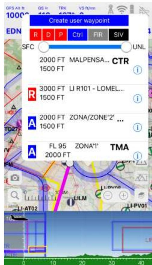
Clicking on an area in the list will temporarily highlight its boundaries in yellow on the map. On iOS, if the profile view is displayed, the area will also be highlighted in yellow in the profile view.
